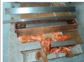
Different straightedge, also for dovetail
