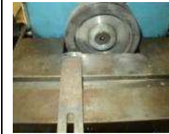
Diamond scraping knife sharpener 5 degrees free angle
