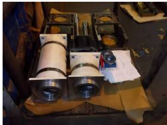
Figure 15: The feed motor was manufactured with an extension and a reduction. WU_232_360
