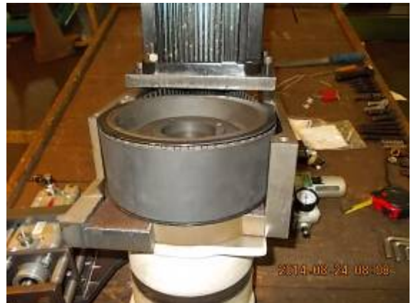
Figure 19: At the Motor Extension, we have made the motor with a rotary flange so that we can rotate the motor in each position. WU_232_400
