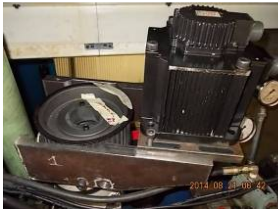
Figure 17: The X motor 1/3 stocky with 3 KW. The old engine had 7 kW and was 1: 1. However, only 10 M Rapid with a 10-er ball screw. WU_232_380
