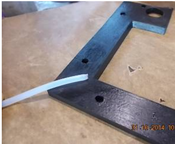
Figure 49: Additional lubrication points for the Z-axis. Normal makes a good mechanical engineers in short-stroke machines more lubrication points in the traverse axis. Mega Bore made only in the Z axis. Now, if ever thread is cut with a moving stroke of less than 200 mm, the long slide with only a lubrication point is lubricated insufficient. We now made three lubrication points per guideway. would be ideal for the long slide 5 lubrication points. But then we would have to dismantle the slide.
