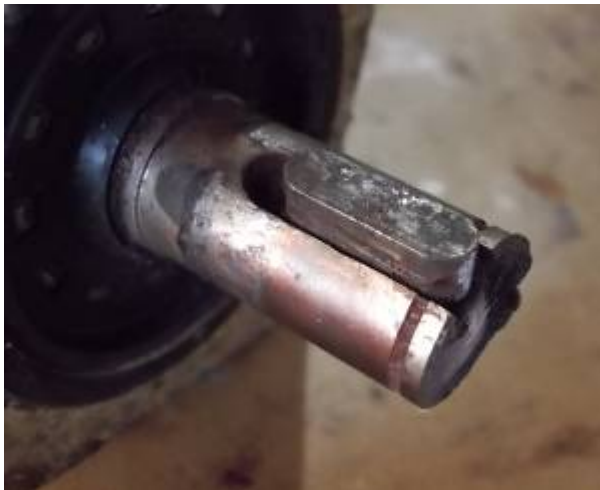
Figure 33: The Fanuc spindle encoder has a lot Pass rust because it was installed without Achsflechterfehler clutch. The shaft and the Pully did not look good. We have installed the encoder with a misalignment compensation. WU_232_270
