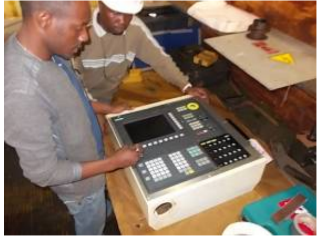
Figure 22: Yoba builds the Sinumerik a 802nd The front plate was made from stainless steel. The thread cutting in stainless steel is more difficult than in normal structural steel. WU_232_160
