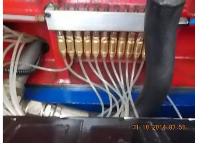
Figure 47: New Dossier unit for controlled lubrication. The CNC lathe Mega Bore simply pumped oil, without volume control. The X axis got too much oil, the Z axis far too little. That is why now spindle already again broken the second Kugelroll-. It sounds like a tractor transmission.
