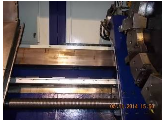
Figure 51: The more oil came, the more abrasion of the sliding coating came out because it ran dry a long time.
