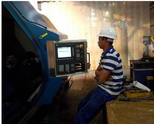
54: And then Carlo Aurujo the CNC is turned on, let PLC program in and completed the commissioning. We all have 110-volt cable from the panel and only 24 volts DC. This has the advantage that the personal injury, as well as lightening strikes, the damage is reduced. On all previous machines no controls are more failed due to severe weather influences. No heat problems. WU_232_330
