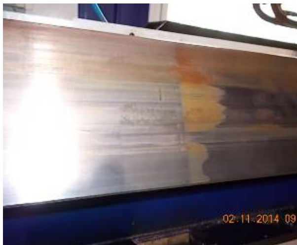
Figure 50: The machine has a faulty lubrication. Only when oil came, the brown sliding coating abrasion appeared.
