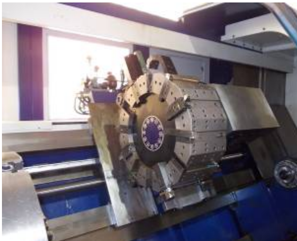
Figure 37: A photograph of the tool turret of the machine without the cover. WU_232_310
