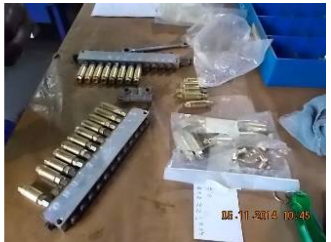
Figure 47: New Dossier unit for controlled lubrication. The CNC lathe Mega Bore simply pumped oil, without volume control. The X axis got too much oil, the Z axis far too little. That is why now spindle already again broken the second Kugelroll-. It sounds like a tractor transmission.
