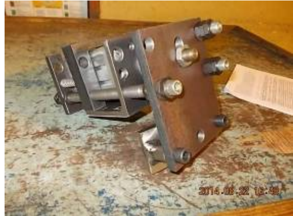
Figure 18: This is the brake construction. This was originally in the engine. We now have the same engine on all CNC machines, so we wanted to order any engine brake. WU_232_390
