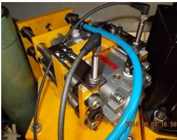
Figure 41: brake cylinder. The cylinder is used as standard.
