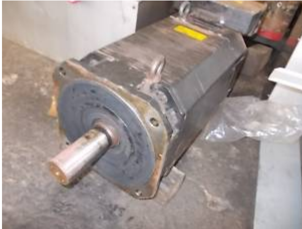
Figure 12: The Fanuc spindle motor seen in Angola after a short period of use very battered. The climate is very angriffig here it verfrisst almost all products.
