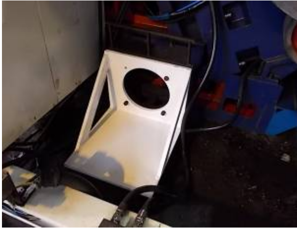
Figure 20: The new engine is a foot motor. We had to make a stand hole. Because of spare parts we use the same type of engine on all machines. Which is in some over-sized, but there are thus virtually never a machine downtime due to lack of spare parts. WU_232_140
