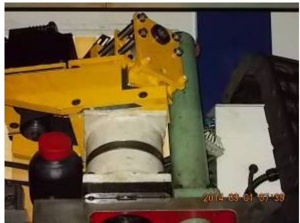
Figure 39: The X motor with the new brake. The brake was made, so that everything can be used the same feed motors.
