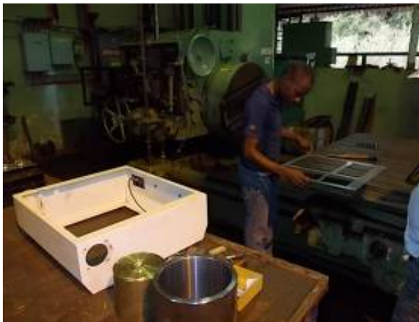
Figure 21: Panel remodeling in preparation. The old Fanuc was dismantled here and we build here is the new Sinumerik 802 DSL pure. WU_232_150
