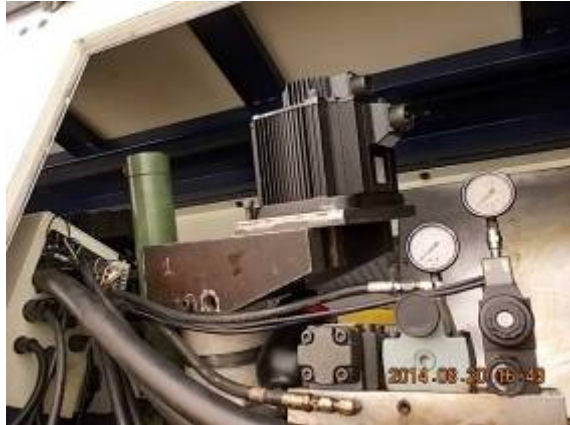
Figure 16: X motor mounting. A very complicated construction, because we have limited space. WU_232_370
