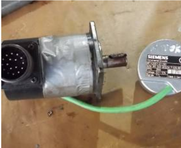
Figure 32: The old Fanuc encoder is missing. A new one is installed. WU_232_260
