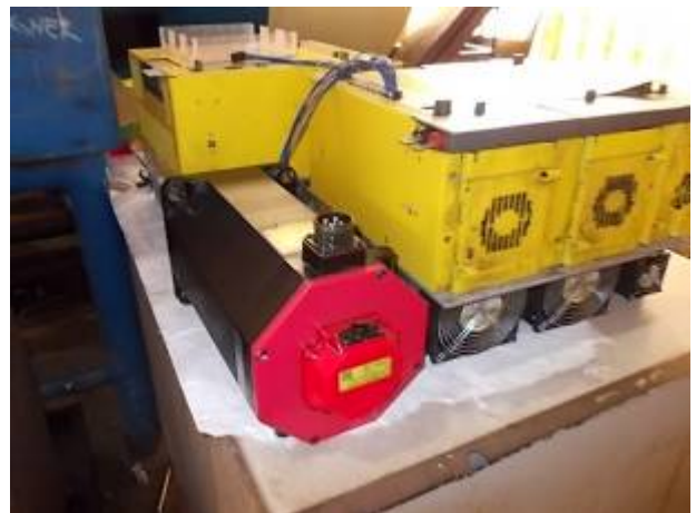
Figure 11: The Z motor. The X motor has a brake. WU_232_110
