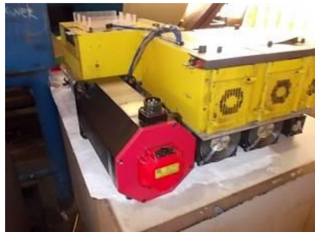
P11) The Z-motor. The X motor has a brake. There are 7 KW feed motors.
