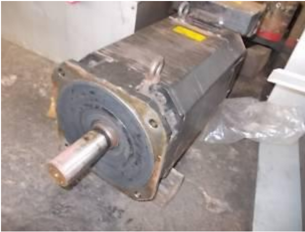
P12) The Fanuc spindle motor seen in Angola after a short period of use, very battered. The climate is very strong here. Impellers crumble in the rule.
