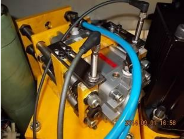
P37) Robust, proprietary brake construction. Braked with switch and unrestrained. Set so that a pressure below 3 bar is detected.
