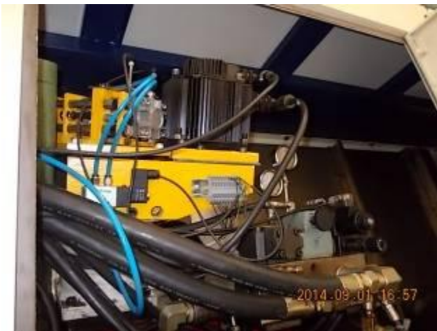
P38) Little space for placement at the 60 ° slant bed CNC lathes arrangement.
