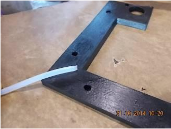
P42) Additional lubrication points for the Z-axis. Normal makes a good mechanical engineer at short stroke machines more lubrication points in the travel axis. Mega Bore made only in the Z axis. If again thread is cut with a moving stroke of less than 200 mm, the carriage is long, inadequately lubricated by only one lubricating point. We now represent 3 lubrication points per track. Ideal would be 5 lubrication points for the long carriage. Dch then we would have to remove the slide.
