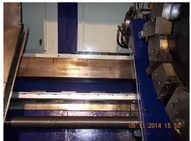
P46) The more oil came, the more wear of the sliding coating came out because it ran dry a long time.
