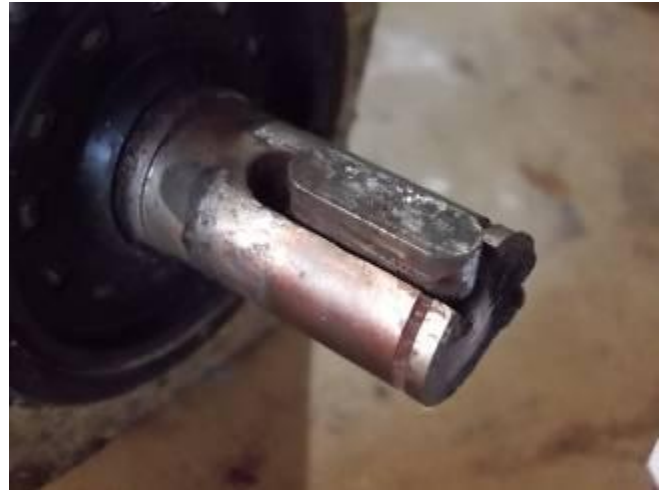
P27) The Fanuc encoder has much fretting because it's mounted without Achsflechtfehler clutch. So how do we do it with the donors that we build on the Siemens CNC.
