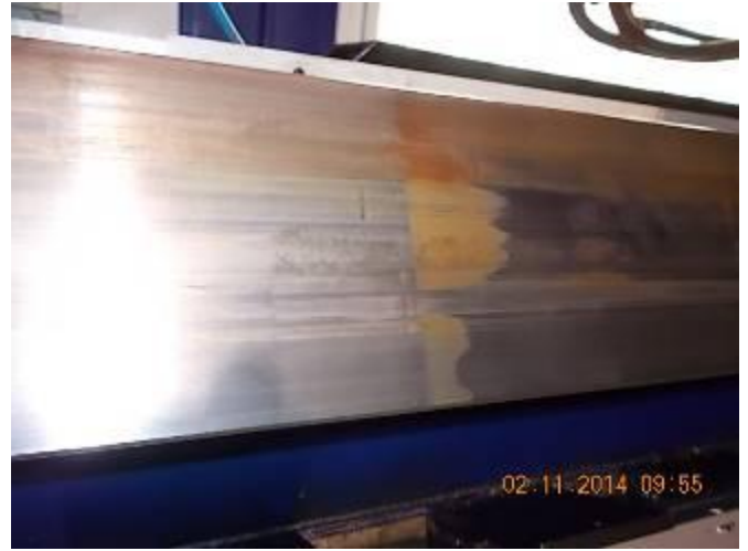
P39) The machine has a faulty lubrication. Only when oil came, the brown sliding coating abrasion appeared.
