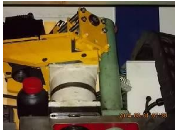
P34) The X motor with the new brake. The brake has been made so that all the same feed motors can be used.
