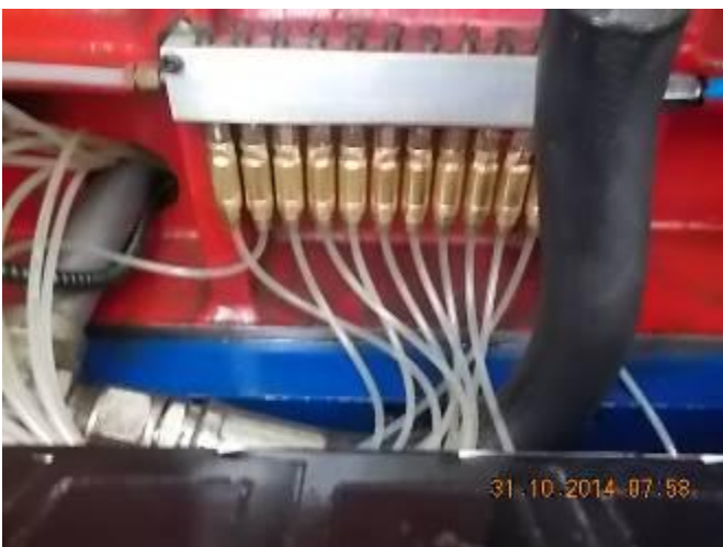
P44) New Dossier unit for controlled lubrication. The CNC lathe Mega Bore has just oil pumped, without volume
