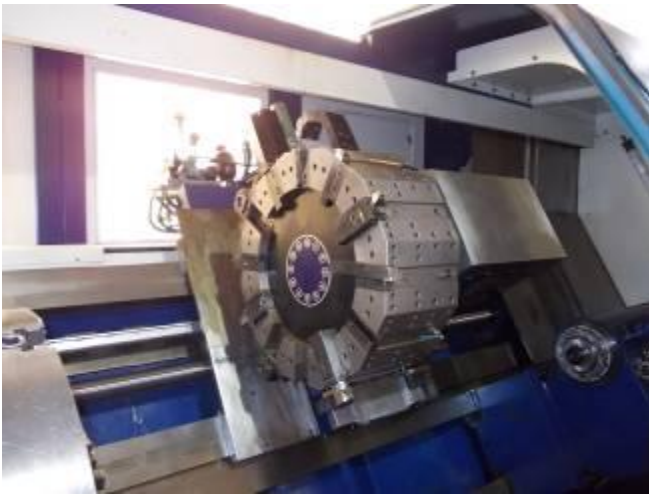
P31) A photo of the turret of the machine without cover. It is an Italian turret Baruffaldi.
