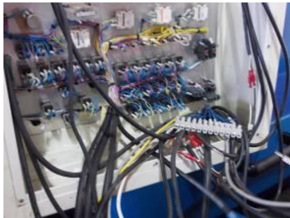
P4) Interior of the old panel. It is remarkable that here a 50-pin cable connects to the front CNC CNC rear. We will replace this with a Profibus cable, 2-pole.
