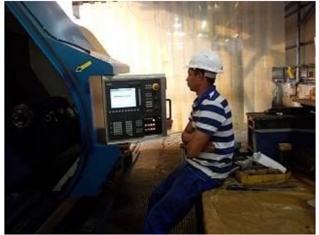
P33) And already Carlo has the CNC off: We all have 110 volts from the panel and have only 24 volts. This has the advantage that no one should expect an electric shock.
