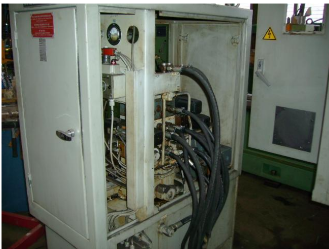
Figure 11: equipped with hydraulic much on the machine. Tailstock, chuck, bezel, Pinole and the whole turret clamping.
