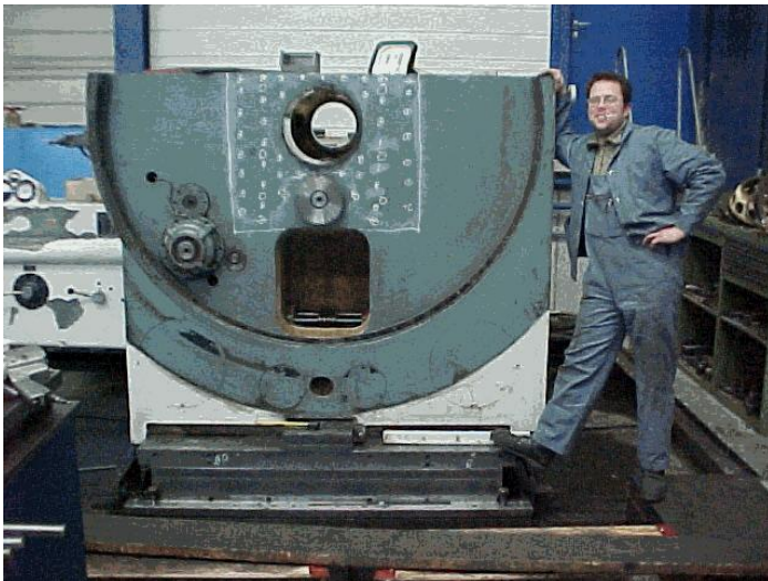
Figure 4: Here we have marked out as we attach a new front panel. The headstock had split a crack across. With the large front panel we have prevented the further spreading. On a boring everything had to be milled clean and many large threads were needed to enable the pressing force coincides with the friction to continue loading large workpieces.
