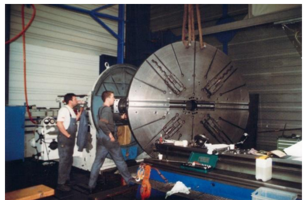
Figure 2: It takes a delicate handling by crane when a face plate must be removed from the spindle nose like that.
