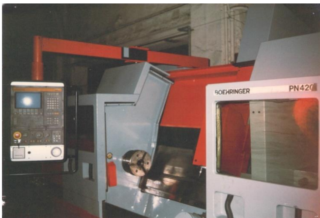
Figure 1: Boehringer PN 420 rebuilt with a new Sinumerik CNC control
