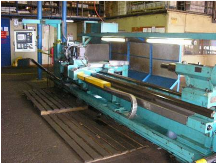
Figure 1: CNC lathe, which was in Switzerland for large company. First CNC was a Sinumerik 5T. This was 20 years later, converted the first time a Sinumerik 810T and a second time a Sinumerik 802nd
