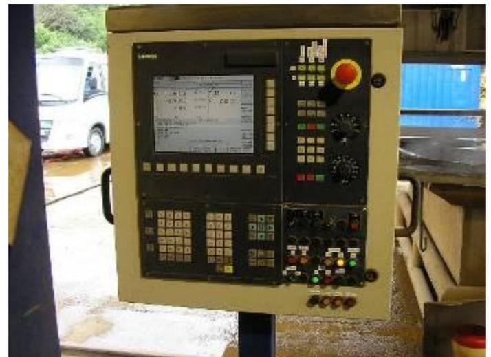
Figure 2: The CNC Sinumerik 802. Designed with Protection levels for various people that not the apprentice may be the same drive with the axes. Or that can program the operator. The machine 7 has protection levels.
