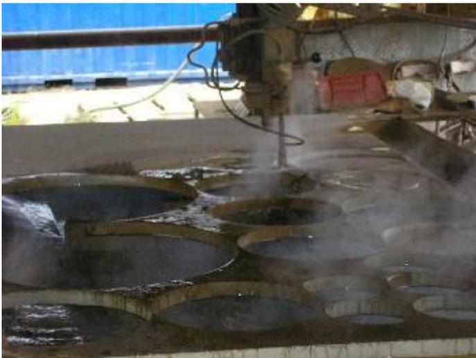
Figure 4: The machine in production. In 0.1 mm Area it cuts steel, aluminum, steel, etc. Importantly, there it must every 6 months the guides above be cleaned, lest the sand from Abrasively cut jerks caused.
