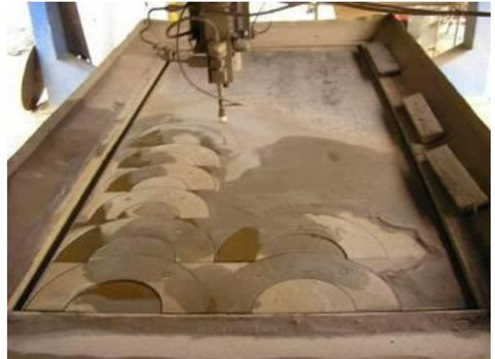
Figure 5: This is where the work of the water jet machine. It can x 4 meters edited plates 3 become. Above all, it needs this machine the stainless material because to do that with the (Q xy Cut) can not flame cutting machine.
