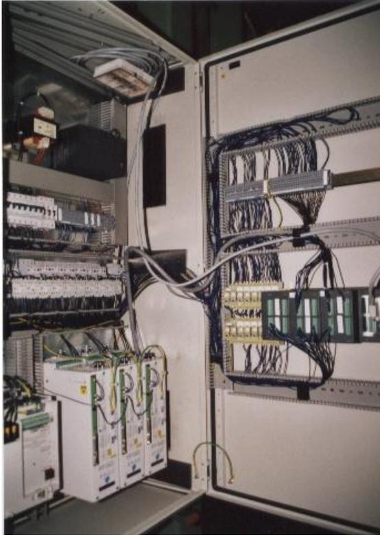
Figure 3: The new electric cabinet by its sides remain on the machine, very easy for transport without disassembly possible. The old large electrical cabinet, the side of disposed of the machine, was disposed of.
