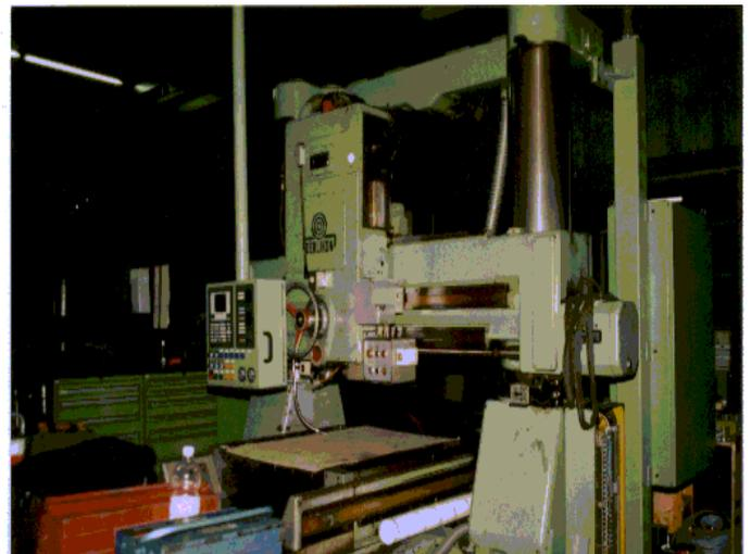
Figure 2: Machine after reconstruction with the new Sinumerik CNC control
