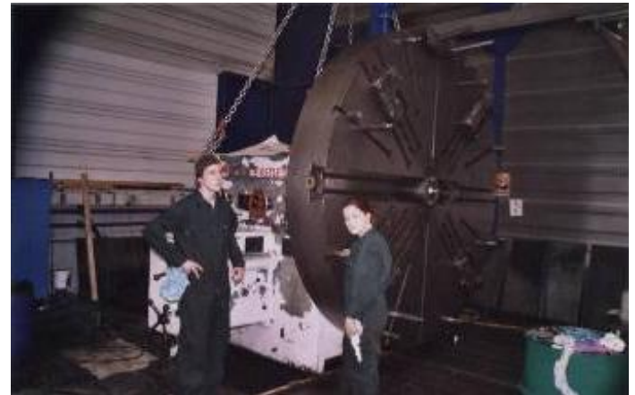
Figure 2: Removing the heavy Heyligenstaedt headstock. It took particularly great tool for the release of the headstock.
