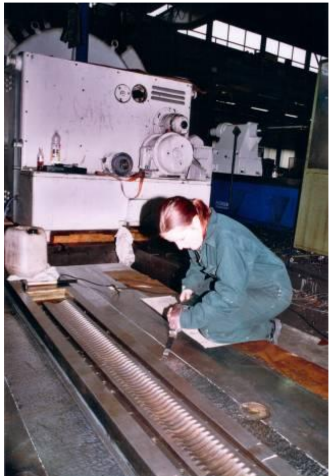
Figure 6: Now the problem with the shaving machine has been corrected. Usually about 0,002 to 0,005 mm per Schabdurchgang, depending on the pressure away. That is, when an error in the 0.1 mm range is, but it must be scraped some.
