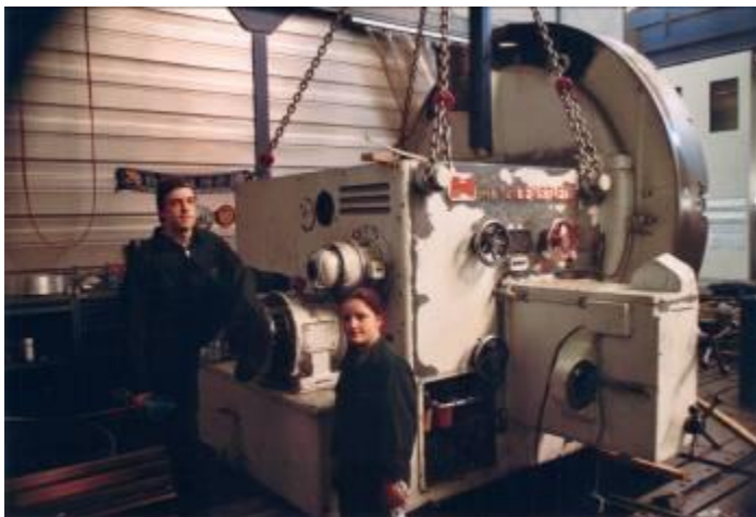
Figure 5: It's to hang the headstock just as with ropes better with the chains. A manufacturer usually makes a Hängejoch, which leaves much just hang the headstock. However, this is difficult in sporadic repairs.
