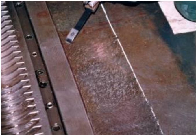
Figure 9: The basic training for scraping the WIAP people have acquired at the company Georg Fischer. At that time, had to continuously scrape be learned 3 months. This knowledge has been incorporated in the WIAP AG into the teaching program.
