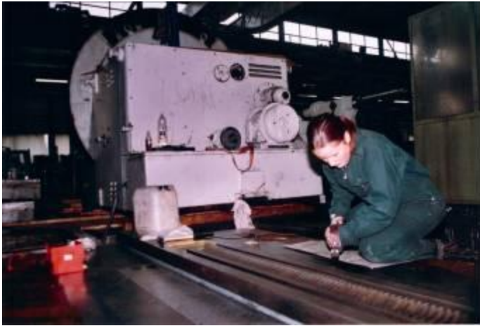
Figure 8: The shaving machine can be scraped about 5 times faster than with the simple hand scraper. A lot of experience exists, it is faster to 20 x.
