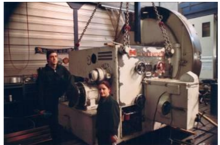
Figure 3: The headstock was raised with chains.
