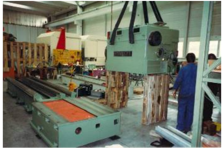
Figure 11: This sturdy, heavy, conventional roll lathe is being rebuilt from the WIAP on CNC. WU4725
