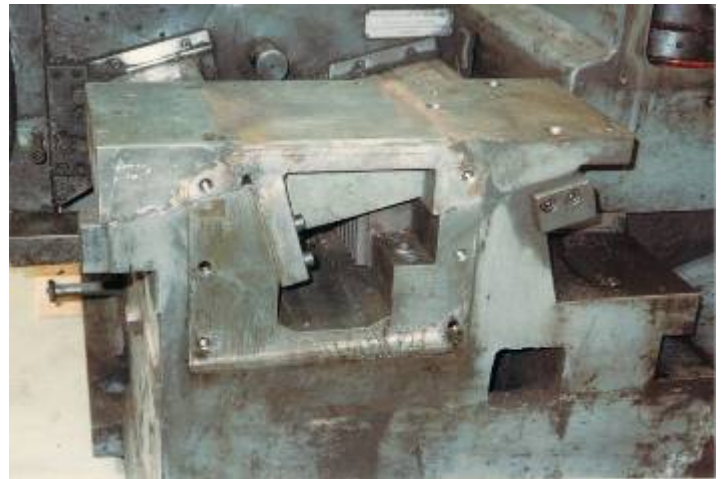
Figure 7: Good, heavy cast, so this machine is not to come to a natural resonance. WU4755
