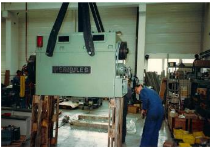
Figure 12: After the grinding bed, the alignment of the machine follows. WU4720
