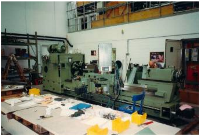
Figure 14: This heavy, robust roll lathe after reconstruction, ready for the return delivery to the German steel mill. WU4775
