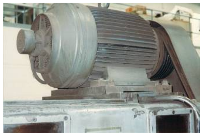
Figure 3: Strong spindle drive motors. The hard roll machining needs a good turning moment. WU4760
