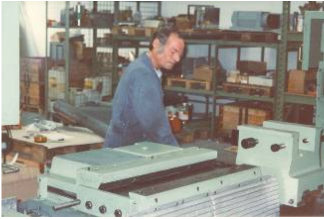
Figure 8: We have improved after-the whole slide system. Lubrication holes completed. All newly sanded and eingeschabt. 10 Pad points per mm 2 inches respected /. WU4730
