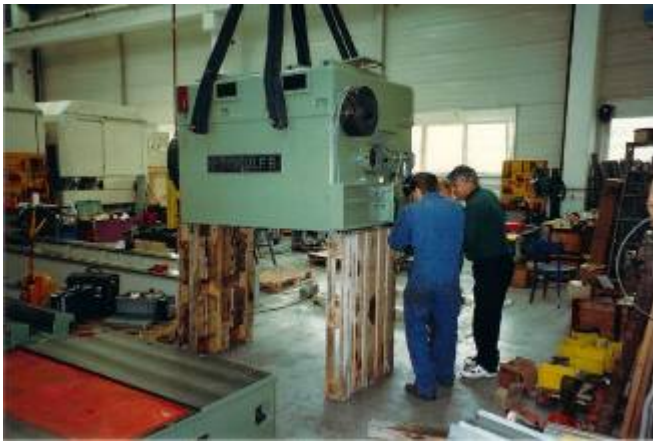
Figure 9: Even the headstock had to be eingeschabt and aligned. Cylindricity of less than 0.02 mm to 500 mm. WU4710
