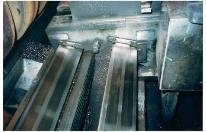
Figure 6: The Z-axis guide is designed for a very strong cross-shaft cutting pressure. The machine had four steels, which simultaneously turned the roll contour. This resulted in a very large management burden. The machine had insert strips made of spring steel, which we shared. WU4740
