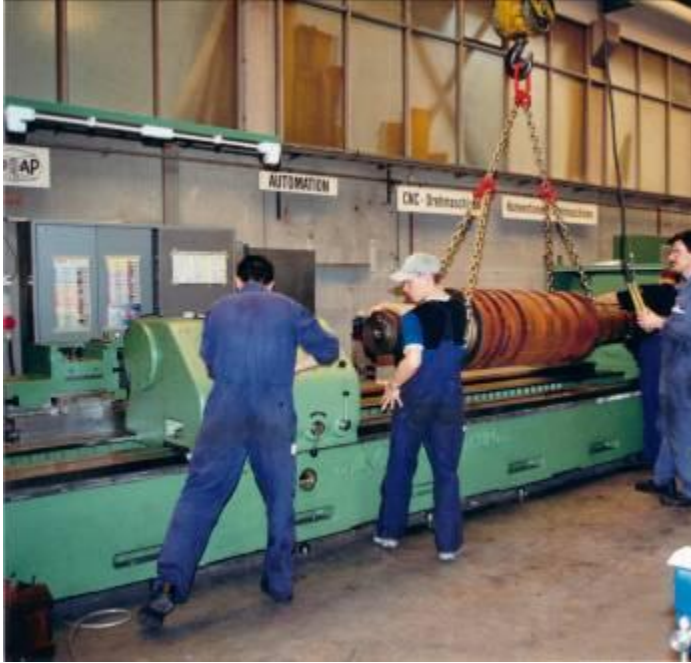
Figure 11: The machine during the rolling test turning. The Z ball screw with 80x10. Covered thanks to the WIAP ball screw capping system.
