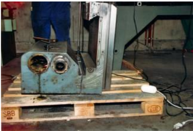
Figure 5: Soon it was the drilling work which goes with a good magnetic drill, done.
