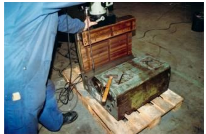
Figure 3: Many holes drilled right next to each other that all just one stroke could be separated at the end. In the cast iron is very good.
