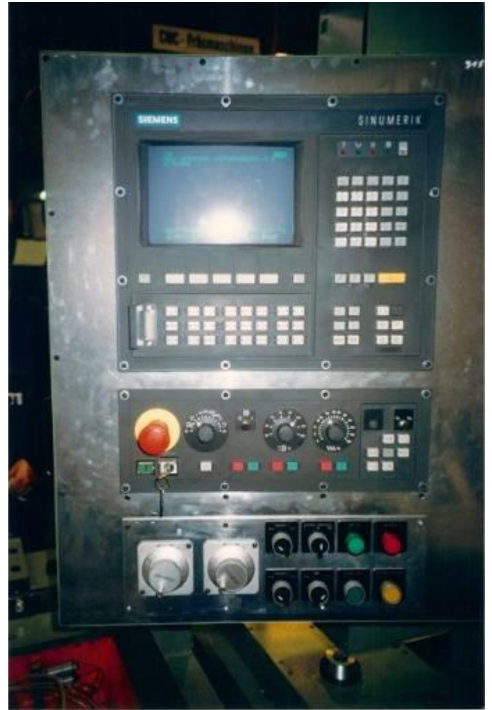
Figure 9: The CNC Sinumerik 810T was made easy to use for operators. Almost no switches were needed to be able to work with the machine.
