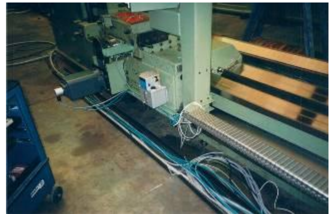
Figure 7: The bed track guide, insert tapes were replaced. The longitudinal slide made new with cable tow. redesigned the entire feed system and renewed.
