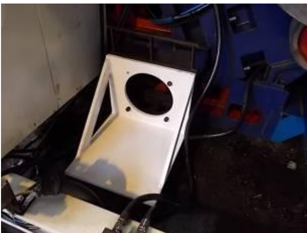
P14) Since the new motor is a motor foot, we had to make a standing frame hole. We install the same engine on all machines. Thus, the spare parts inventory is easier.
