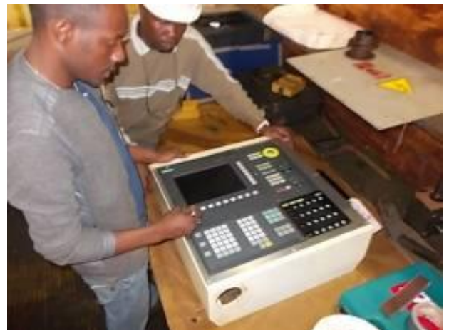
P16) Yoba builds the Sinumerik 802. The front plate is made of stainless steel. The boys realize that tapping on stainless steel is persistent.
