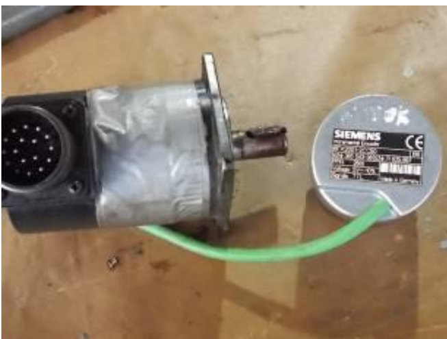
P26) The old Fanuc encoder (left) is coming off. A new (right) is mounted.
