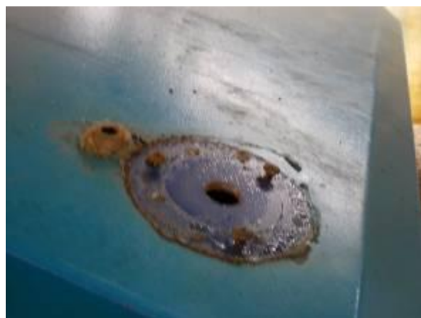
P1) That was a lamp. Above where the screw was a hole. That was the reason why the CNC Fanuc 18 i was destroyed.
