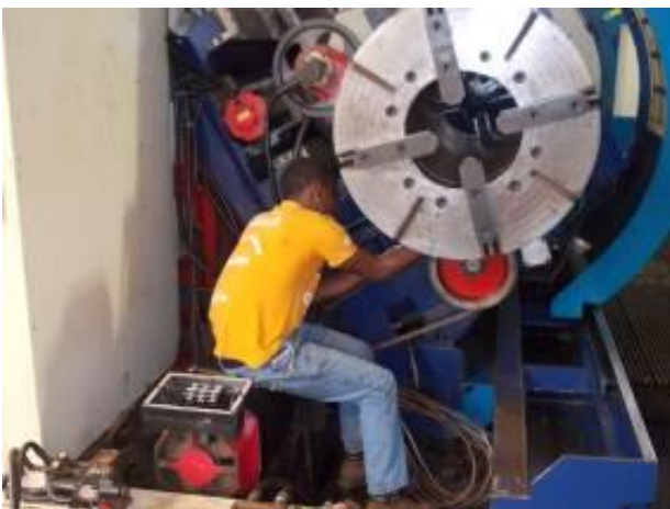
P13) Yoba in the development of the main motor. He removed the V-belt.
