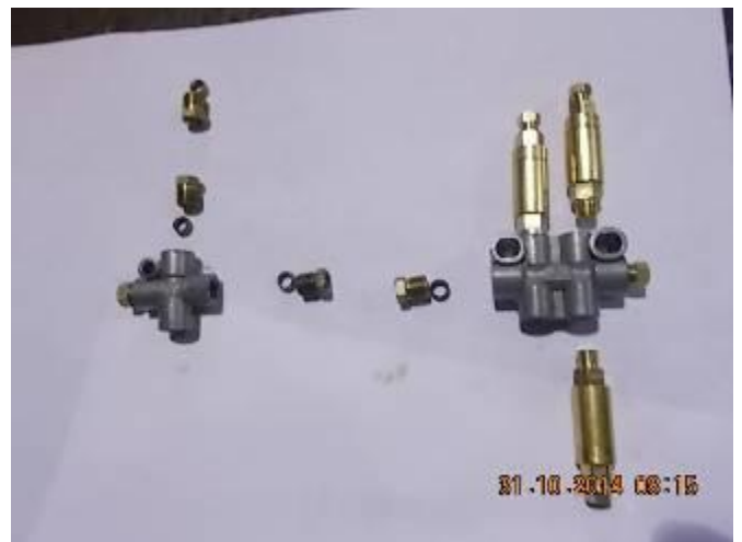
P41) Lubrication tag. The ball screw gets a double quantity of oil.
