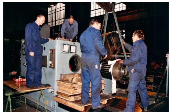
P7: The gears and shafts camps were at the Maschie all fitted with the SKF Press Association disassembly and re-assembly demanded some effort.
