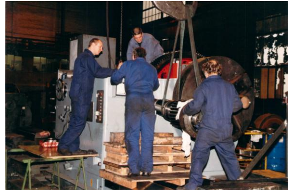
P6: The headstock was also revised, there were some gears defective. Messrs. Walter Grell made at the time the gears according to pattern.
